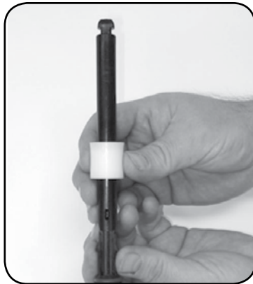
Step 4. For 5% Replace #44 DOSAGE PISTON flared-end up and #14 O-ring. 0.3% only: Replace #51 SHAFT ASSEMBLY. See Step 5a.
